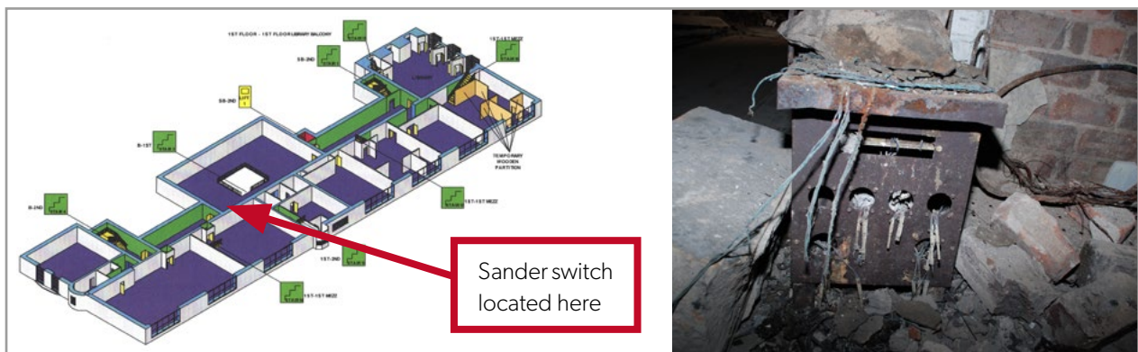
Figure 20 – Location of floor sander switch and the remains of one of nine 110volt site transformers
