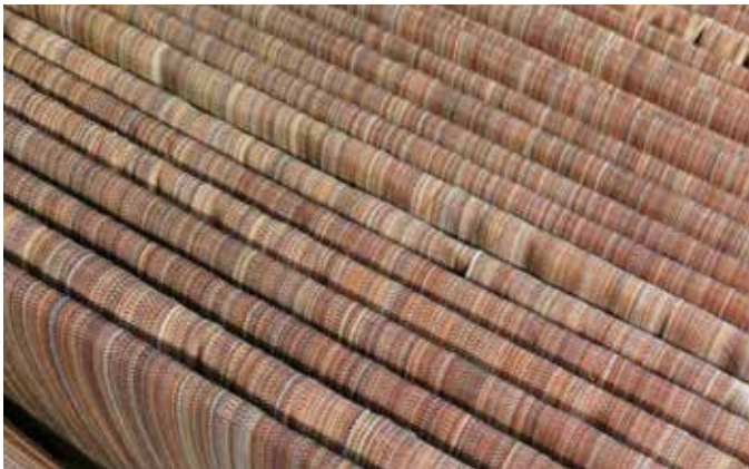
Fig. 13 The walls of the billiards room were lined with horse-hair padded panels. The recreated panels were made with contemporary horse hair sourced from John Boyd – one of the last companies in the world still weaving it. (Top): The horse hair is cut to size before (lower): being wrapped over padded boards to create the wall panels. Image (lower): © John Cowie
