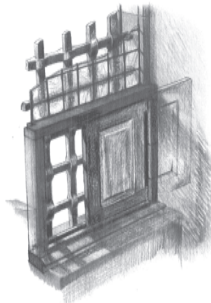
5. Baltersan : conjectural reconstruction showing how the shutters slid within the thickness of the 1.25 metre-thick wall.
